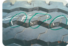
Tire Crown Pattern Breaking Damage
