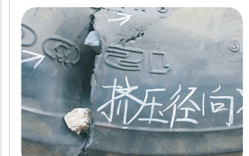
Foreign Material Between Side Wall
