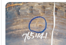
Side Wall Scratch
