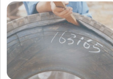
Puncture and Delamination
