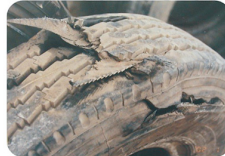
Tire Crown Impact Blast
