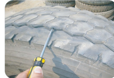
Tire Crown Abrasion Under Low Air Pressure
