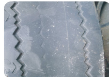
Tread Wear Under High Air Pressure
