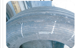
Shoulder Damage & Pattern Block Dropping Off
